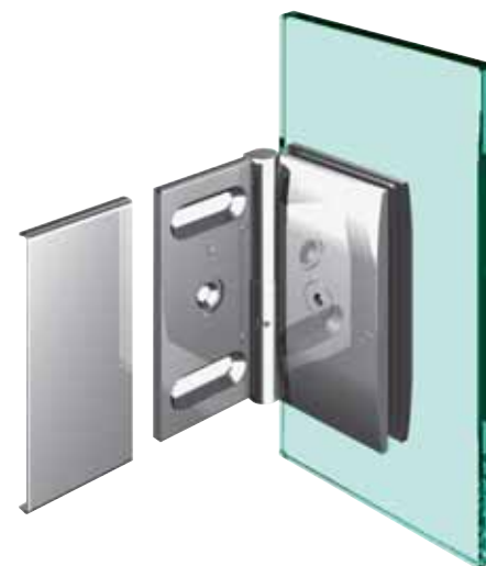
Winkelverbinder Glas-Wand 90°, Gradzahl stufenlos von 60° - 100° verstellbar/corner bracket glass-wall, 90°, Degree of angle is infinitely adjustable between 60° and 100°, Art-Nr.: 8430MS
